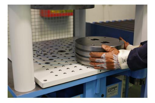
The machine allows to assemble die plate and mandrel, by eliminating also the annoying noise pollution caused by hammer work. This is why Compes has designed a high-tech system that is composed of three main elements:
